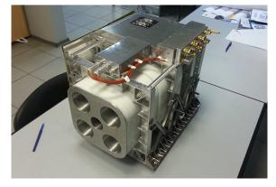
1 neutron detector 0.4 eV - 500 keV 1 neutron detector 0.5 MeV - 10 MeV
