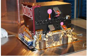
1 UV-VIS spectrometer: 0.2 - 0.65 μm 2 IR spectrometers: 2.2 - 4.3 μm
