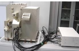
1 NIR spectrometer: 0.7 - 1.7 μm 1 MIR spectrometer: 2.2 - 4.4 μm 1 TIR spectrometer: 1.7 - 17 μm
